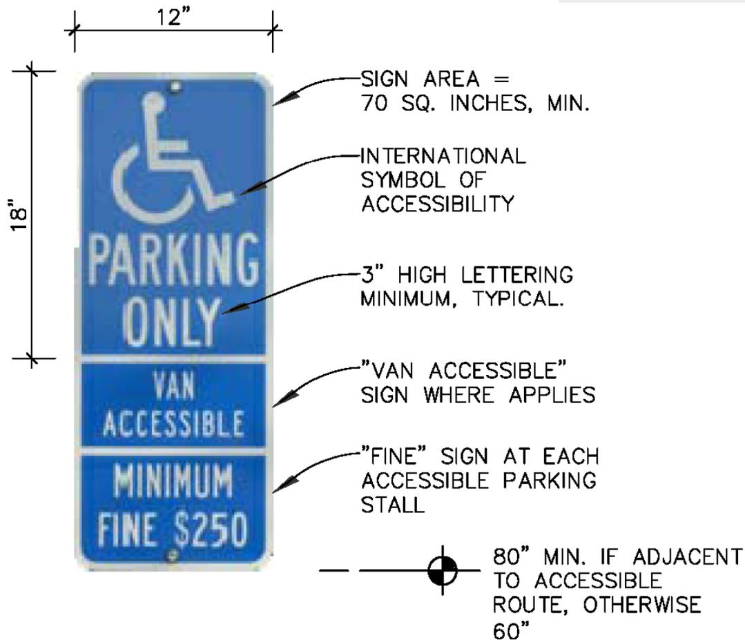
Sign placed at the end of the parking stall on pole or on wall of building
