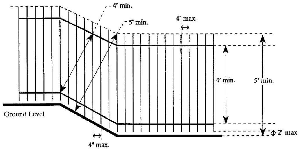
Figure 31B-4 Perpendicular fencing dimensions on sloping ground.
