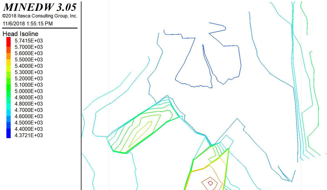
Figure 1. Head isolines extracted from the steady-state Lone Tree simulation.
